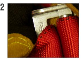
The manufacturer's name (identified as PenSafe or PS) and three-digit manufacturing code will be covered. Push web to the side to reveal the stamped markings.
