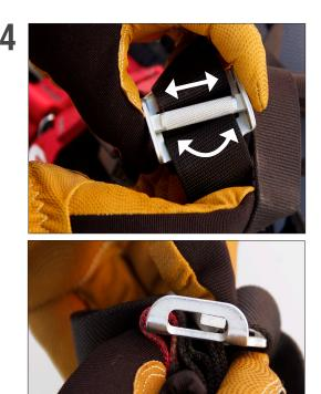
With access to the buckle, move the friction bar in all directions—up, down, side-to-side and diagonally—to ensure it does not separate from the buckle frame.
