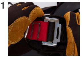
Locate and identify the PenSafe Friction Buckles on your harness / strap.
