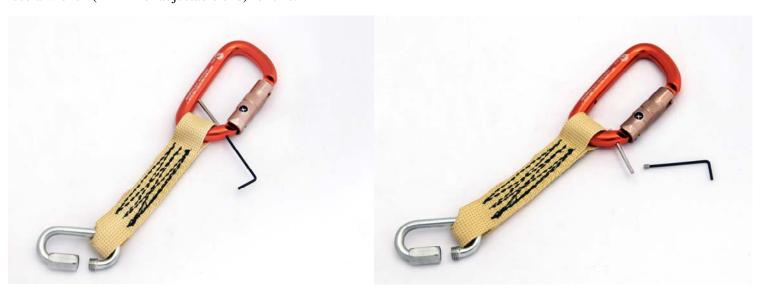
2. Using the included 5/64" hex wrench, remove the set screw and keeper pin from the carabiner in the original tether. Occasionally the keeper pin gets pressed in fairly tightly, so you may need to loosen it with pliers to remove it.
