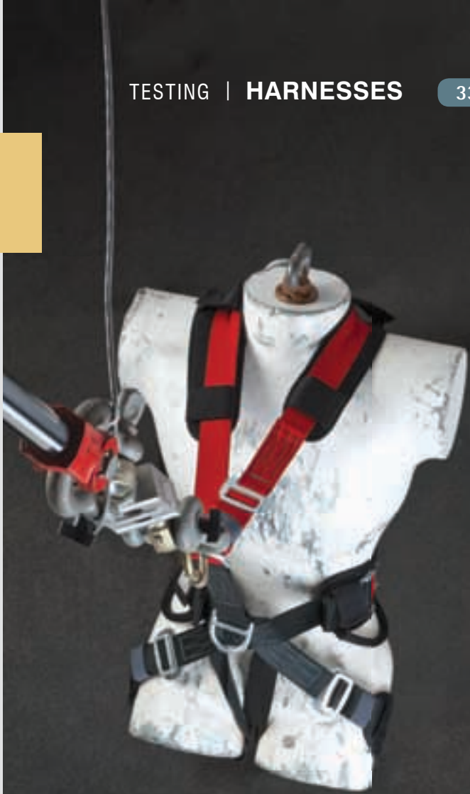
Static test of a CMC Fire-Rescue Harness on a 300-lb. test torso.
