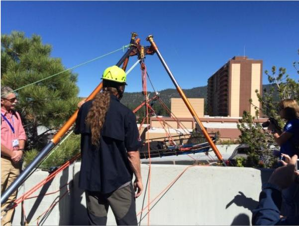
PMI ([www.pmirope.com](http://www.pmirope.com)) demonstrated a deflection line raising and lowering system using the SMC/Skedco/PMI TerrAdaptor portable high directional anchor system. PMI and SMC staff utilized the mechanized Harken PowerSeat on PMI's Extreme Pro rope for the raise and lower of the Cascade Rescue two-piece titanium litter.
