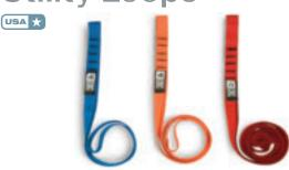
Designed for placing protection when climbing towers, our Utility Loops allow versatility in setting anchors. Sewn from 1-in. (25-mm) mil-spec tubular web for high strength and good grip when tied off with a girth hitch, MBS (loop) is 31.1 kN (7,000 lbf.).
