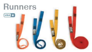
Made from 1-in. (25-mm) mil-spec tubular web, these runners have a loop sewn at each end. Available in four sizes that have proven popular for rescue operations, the large size works well for tying a mariner's knot. MBS end-to-end is 16.9 kN (3,800 lbf.).
