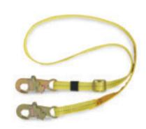
This lanyard has self-locking snaps at each end and can be adjusted from 4 to 8 ft. (1.2 to 2.4 m). Its 1-in. (25 mm) polyester web has a built-in wear indicator.
