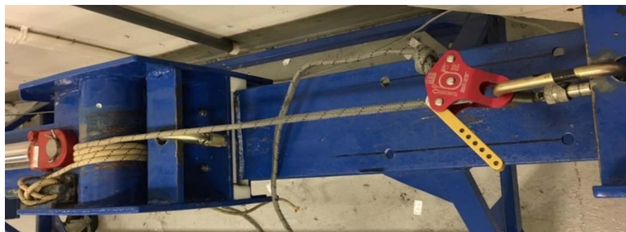
Figure 4 - CMC Horizontal Test Apparatus Testing System Strength
