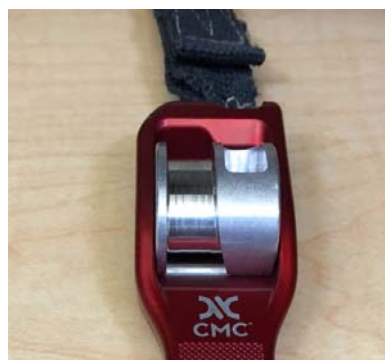
Figure 7 - LEVR device after conditioning cycles
