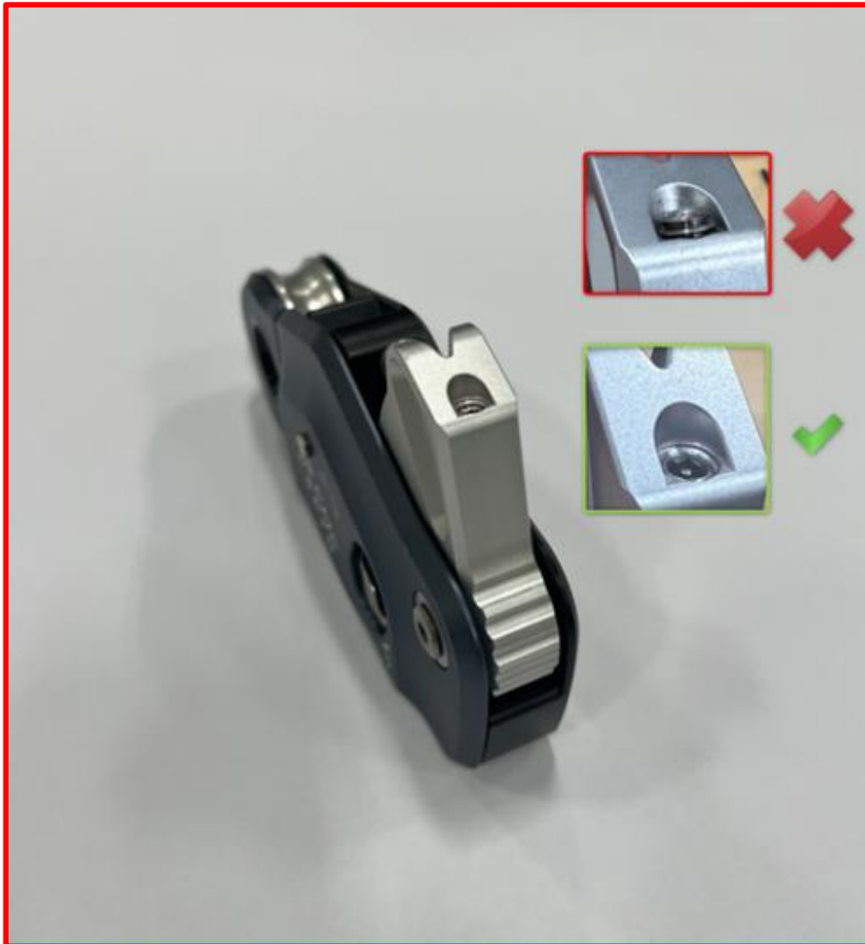
(Figure 1: Correct and Incorrect Cam Screw Height)
