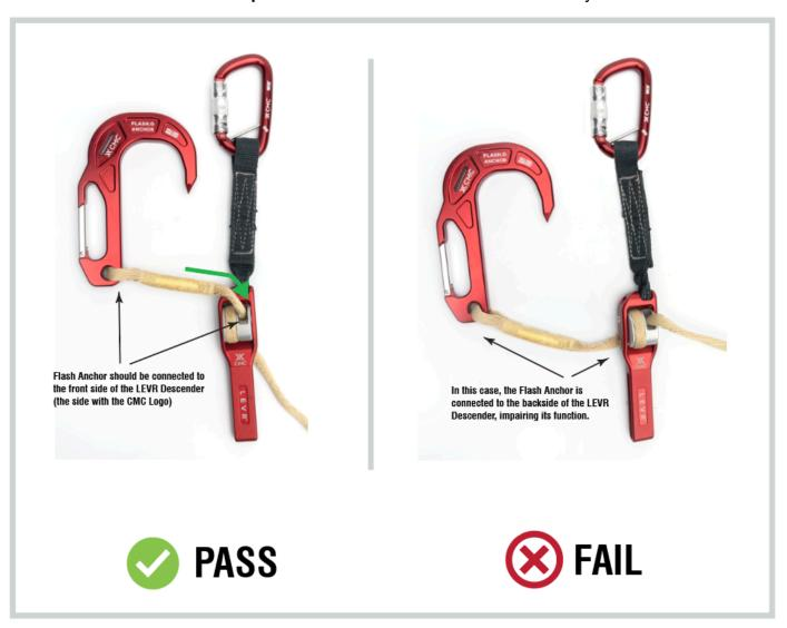
**Inspection Procedure:** Hold the LEVR Descender with the CMC Logo facing you. Does the Flash Anchor connect to the front side of the LEVR Descender? No = system fails inspection.
