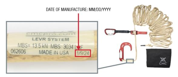
Remove your LEVR Escape System from service if the manufacture date is between January 1, 2023 and February 1, 2024 and follow inspection procedures below. As a reminder, all LEVR Escape Systems should be inspected and function tested before/after use and yearly in accordance with the <u>User Manual</u>. 3. Inspect your LEVR Escape System for proper reeving of the LEVR Descender. Refer to the images below for specific examples of passing and failing inspection.
