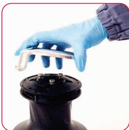
4. Remove the self-tailing arm by rotating and lifting it.
