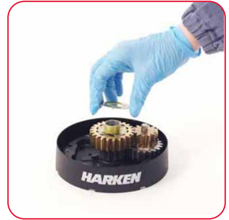
12. Remove the washer. Important: washer may remain inside the drum support!
