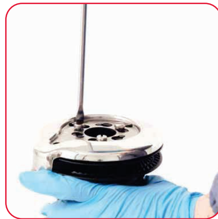
3. Unscrew the three screws (4Nm/35in-lb)
