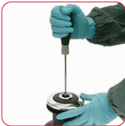
1. Unscrew the central screw (2Nm/18in-lb)
