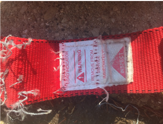
Fall arrest indicator that has been deployed
