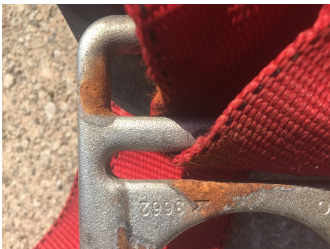
Corrosion on the attachment point
