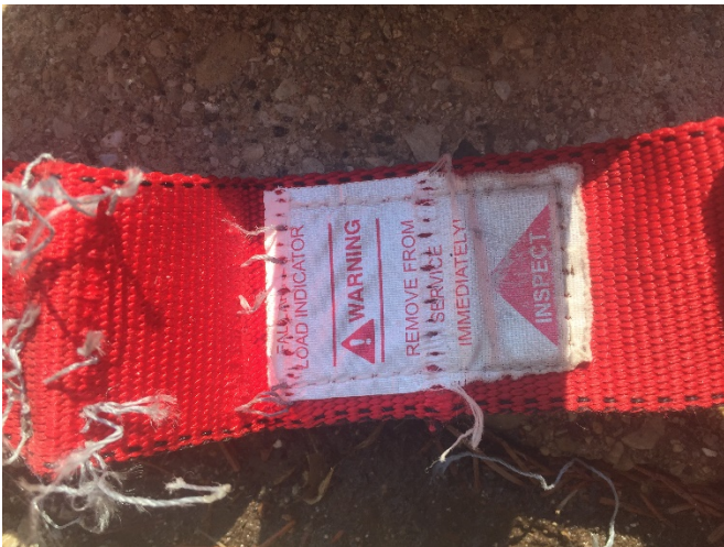
Fall arrest indicator that has been deployed
