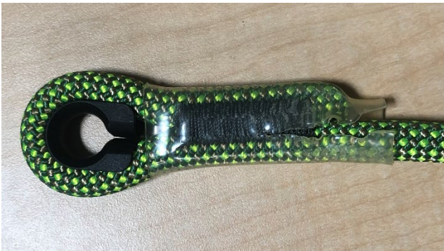
Damaged Protective shrink tubing.
