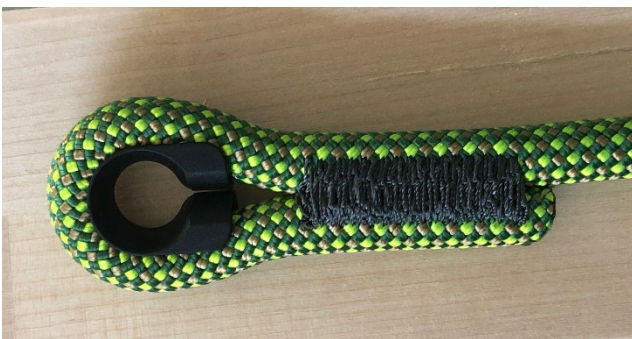
Missing protective shrink tubing, and product label.
