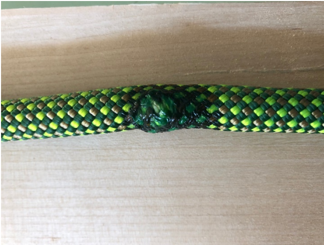
Damage to the rope from excess heat.
