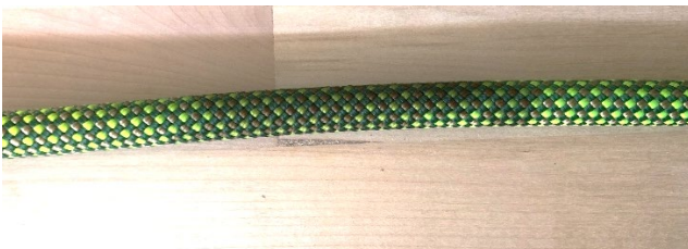
Heavy contamination with an unknown substance.
