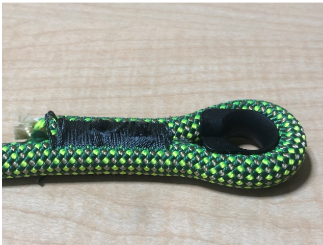
Damaged structural stitching.
