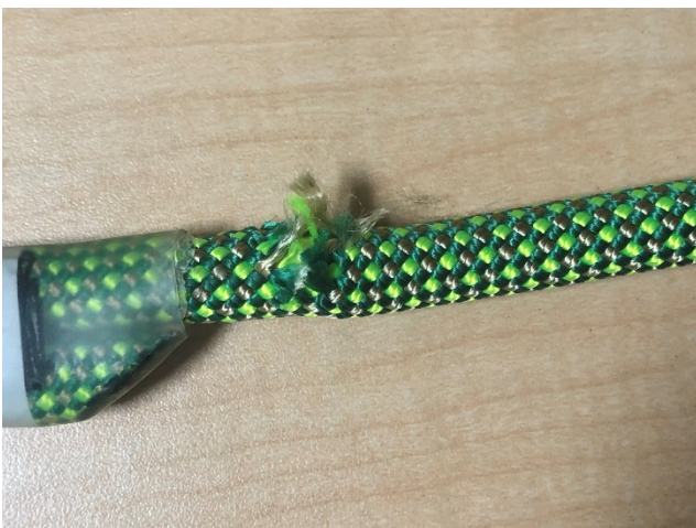
Damaged rope, cuts, abrasion, bulging.
